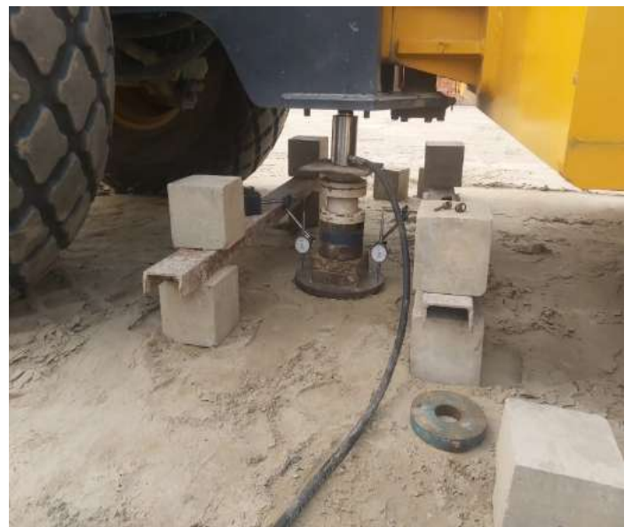
Soil Bearing Capacity checking
