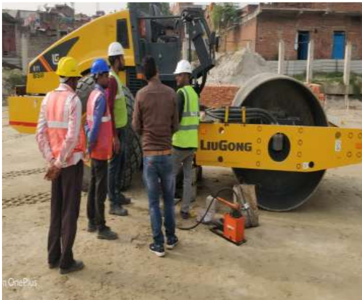
Soil Bearing Capacity checking
