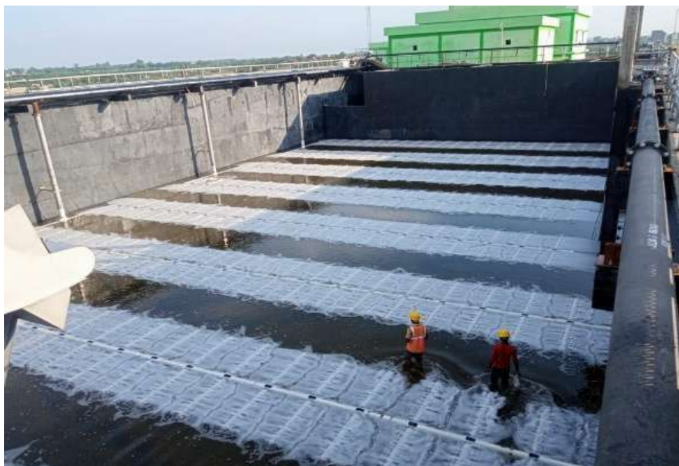
Diffuser leakage testing done
